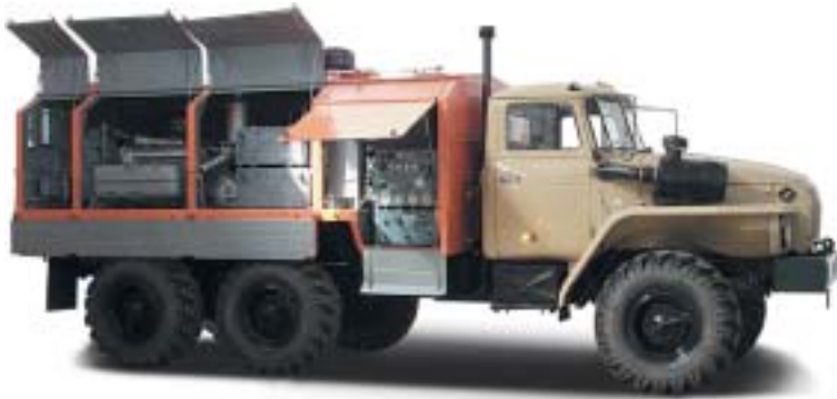
PKS-8/101 mounted on Ural truck chassis
