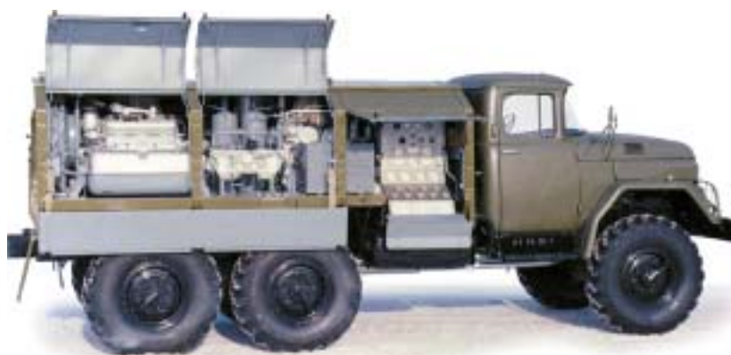
UKS-400V-131 mounted on ZIL-131 truck chassis
